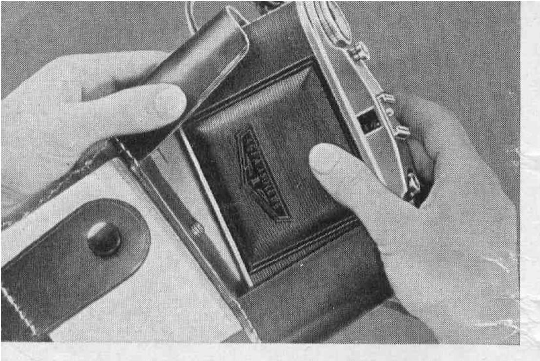
To insert film, unscrew tripod screw of ever-ready case, take out camera.
