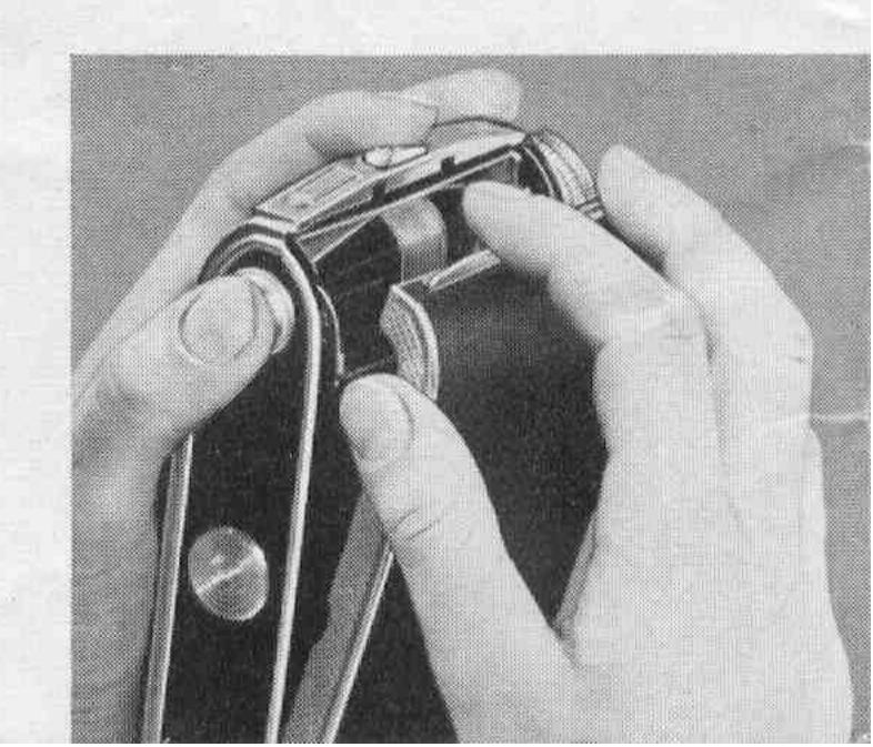
Turn out spool holder, and pull hinged spool carrier outward.
