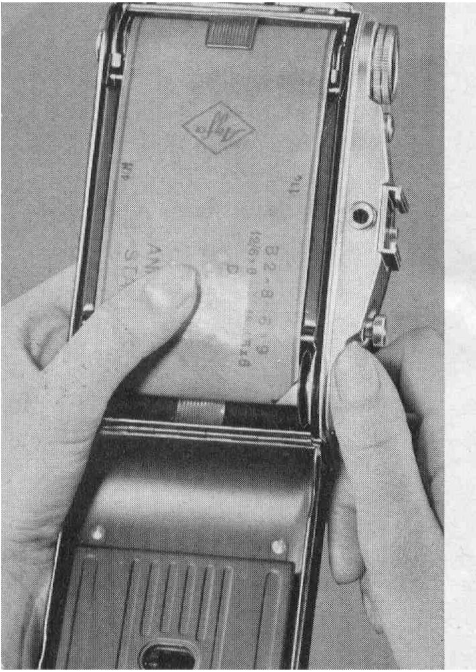
Tear adhesive tape and remove it carefully. Pull out backing paper, and insert it in the longer slot of the spool.
