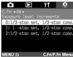
1: Sets full-stop increments for the shutter speed and aperture.
