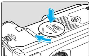
**5** Close the cover by turning it clockwise, as shown by the arrow in the diagram.
