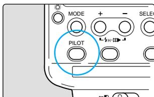
**2** Make sure the 550EX Speedlite's pilot lamp is on.
