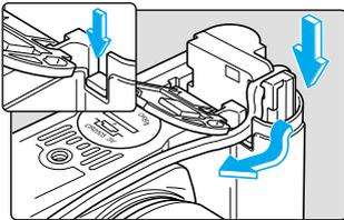
**1** Insert the DC coupler (→29) and set the Main Switch to **⟨ON⟩**. (→31)
