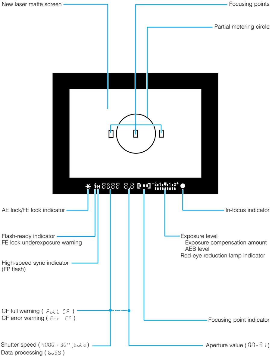
The above diagram shows the LCD panel with all icons and indicators displayed. In actual use, the items displayed differ according to the camera settings.
