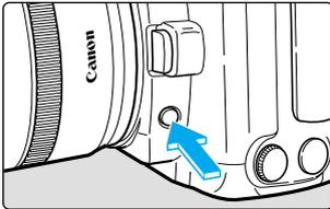
You can press the Depth-of-Field Preview button to close the aperture to the current aperture setting, and then verify the range of focus in the viewfinder.
