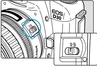
**1** Set the lens focus mode switch to  $\langle AF \rangle$ .
