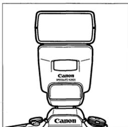
When the 420EX is mounted on a Type-A camera such as the EOS 30/ELAN 7E, using E-TTL autoflash is just as easy as normal autoexposure (AE). E-TTL autoflash uses the camera's multi-zone metering sensor for highly precise flash exposure control. A preflash is fired for evaluative flash metering and the reading is used to determine the main flash output. The result is a flash picture with excellent balance between the flash illumination and ambient light.
