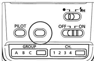
If the correct flash exposure has been obtained, the flash exposure confirmation lamp lights (in green) for about 3 sec. after the flash fires. If the flash exposure confirmation lamp does not light after the flash fires, the picture may have been underexposed. Move closer to the subject and try again.
