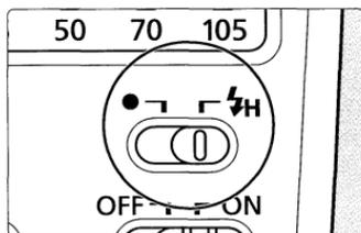
**2** Set the high-speed sync switch to <⚡H>.
