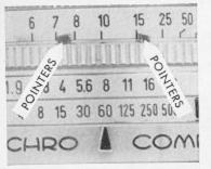
and behind the subject, will also be in focus. This range of sharpness is known as "depth of field." The larger the f/number (smaller lens opening), the greater the depth of field at the same distance setting.
