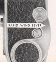
NOTE: When the rapid wind lever is swung out, the rewind knob should turn counterclockwise (after slack has been taken up in the magazine). This will provide a check on whether or not film is advancing properly.
