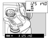
Select this mode when you use a flash. The shutter speed will be fixed at 1/125 second for synchronization. To adjust synchro speed, turn the rear dial.
