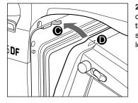
2. When detaching the digital back from the camera body, the shutter will automatically fire, the mirror will go to the upper position and the shutter curtain will open, leaving the camera locked.
