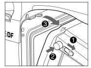
When detaching the digital back, pull back the detachment lever (found on the right side on ZD backs) or press the release button (found on the left side of M series backs) and pull away from the camera body.
