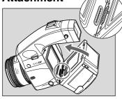
**1.** Align the lower contact pins of the digital back with the lower contact pins on the camera body.
