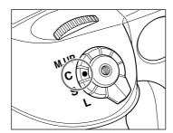
Set the shutter release mode selector lever to "C" and hold down the shutter for continuous shooting.
