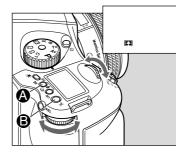
**1.** Exposure mode mark is displayed when the exposure mode button **(2)** is pressed. Since three different exposure modes are displayed sequentially when either the front or rear dial is turned, select an appropriate exposure mode.
