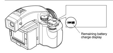
• The camera's power is turned on when the drive dial is set to "**S**," "**C**" or "**M.UP**." In order to prevent the camera's battery power from draining, sleep mode is automatically established if no operations are performed for a specific period of time while the power is ON (with exposure metering status maintained).
