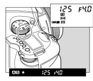
1. Turn the exposure mode setting dial to "**M**" (Manual) position.
