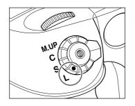
**1.** Turn the shutter release mode selector lever to the "L" position (power OFF).
