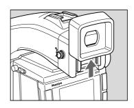
**1.** Remove the rubber eye piece by sliding upwards.
