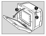
**1.** First remove the protective covers from the camera body and digital back.
