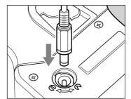
**4.** Connect the external battery case to the body.
