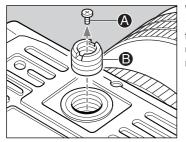
When using a tripod with 3/8" screw (instead of 1/4" screw) remove the small screw () from the tripod screw hole on the bottom of the body using a plus screwdriver, then use a coin to remove the tripod screw adapter bushing ().
