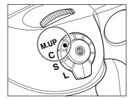
When the shutter button is pressed, the mirror moves up, and when the shutter button is pressed again, the shutter is tripped, and a picture is taken. For the mirror up shooting procedure, see pages 62 to 64.
