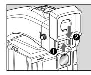
**3.** Insert a new diopter by aligning it to the base of the diopter holder and sliding it upwards into place then reattach the rubber eye piece.
