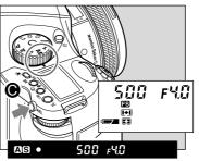
While the difference (a) between the set value (a) and the metered value is displayed on the viewfinder LCD, press the AEL button (b) for approximately one second. The camera changes the shutter speed to an appropriate level.
