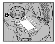
To see the main panel at night or in dark places, press the backlight button ④/深. The backlight will go on approximately 20 seconds and go off unless there is another operation.
