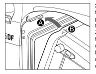
2. Rest the digital back on the lower ledge of the camera body so the camera body contact pins and digital back contact pins meet. Hold the digital back lever open (on the right side of ZD backs) or hold down the release button (on the left side of M series backs) then press the upper part of the digital back () to the camera body (). A click will be heard as the shutter is released, signaling that the back has been correctly mounted.
