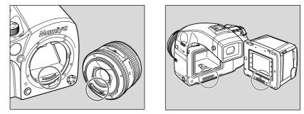
★ Oil, dirt, fingerprint, or moisture on the electrical contacts may cause malfunction or corrosion. Keep the contacts clean with a dry clean cloth.
