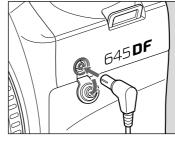
1. To use a grip type flashgun or a strobe with other electric contacts than X contact, connect the sync. cord to the camera's sync. terminal. (See note below about flashes designed exclusively for other maker's cameras.)
