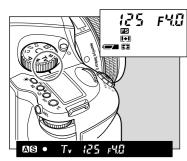
**1.** Turn the exposure mode setting dial to "**Tv**" (shutter priority AE) position.
