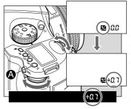
1. When exposure compensation button () is pressed, (2) appears on the external LCD. When the front or rear dial is turned counterclockwise, the exposure is increased; conversely, when it is turned clockwise, it is decreased. The exposure compensation value can be checked on the external LCD or LCD inside the viewfinder.
