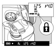
When dial lock is set, the dial lock display " $\square$ " appears on the external LCD.
