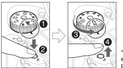
\* The illustration shows the exposure mode "Av" (aperture priority AE) being recorded to C2.
