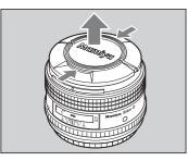
To remove the front lens cap, squeeze the shiny sections together and lift out.
