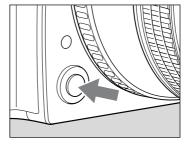
After focusing, press the preview button. The diaphragm will be stopped down to the set aperture.
