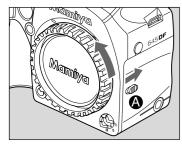
1. Remove the front body cap, just like you would remove a lens, by pushing the lens release button () backward and then turn the front body cap counter clockwise and lift out.
