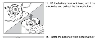
1. Lift the battery case lock lever, turn it counter clockwise and pull out the battery holder.
