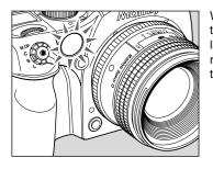
When the subject is dark or under-exposed and the camera fails to auto-focus, a red lamp may light on the front of the camera when the shutter release button is half-pressed. This is a light that assists the camera's auto focus function.
