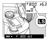
**F5.3** When using the leaf shutter lens, the leaf shutter's working range is from 1/800 sec. to 1 sec. For other speeds (1/4000-1/800 sec., 1-60sec., bulb) use the focal plane shutter.
