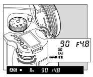
2. Turn the front or rear dial to set the desired aperture.
