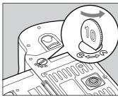
**2.** Use a coin or similar object to turn and remove the external battery socket cap.
