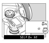
**4.** Turn the rear dial to select the countdown time. 0.5/ 1 sec. to 10 seconds is selectable by the second, 10 seconds to 90 seconds is selectable by units of 10 seconds, 2 minutes to 10 minutes is selectable by the minute while 10 to 60 minutes is selectable by units of 10 minutes.
