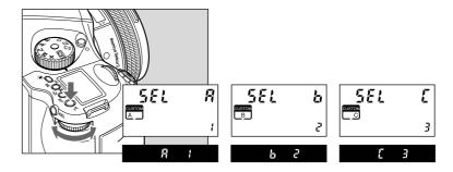
1. By turning the exposure mode dial, "CF" (custom function mode) can be selected.
