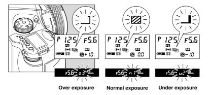
**5.** Press the auto bracketing button (2), then turn the front dial to "DF" to cancel. Then press the auto bracketing set button (2) or half-press the shutter button to return to the normal display mode.
