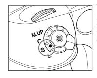
The drive dial has an "**S**" (single-frame advance mode) setting and a "**C**" (continuous advance mode) setting. (See page 42.) When set to "**L**," the power is turned off. When set to "**M.UP**", the mirror moves into the set postion.
