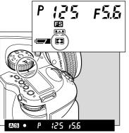
There are three exposure metering modes: In the "**A**" mode the average brightness in the entire frame is measured with emphasis on the center of the frame. The brightness at a specific spot in the center of the frame is metered in the "**S**" mode. The "**A-S**" mode automatically switches between these two modes depending on the contrasts in the picture. (See page 54.)
