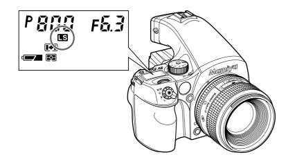
When the leaf shutter lens is attached, the letters "**IS**" will appear in the main LCD display. (The leaf shutter icon will also appear).
