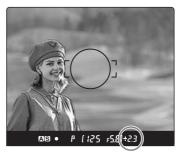
Keep pressing the AEL button (a), and the difference between the metered exposure value and the exposure of the new composition will be displayed on the viewfinder LCD. This function can be used to see if an object of very different brightness levels can be properly captured.
