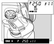
Turn the exposure mode setting dial to "**P**" (program AE) position.
