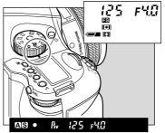
1. Turn the exposure mode setting dial to "Av" (aperture priority AE) position.
