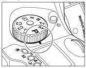
There are four exposure modes: "**P**" (program AE), "**Av**" (aperture priority AE), "**Tv**" (shutter priority AE) and "**M**" (manual mode). "**X**" is for synchro mode, while "**CF**" is used to for custom functions.
