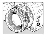
While sliding the lens release button back (), rotate the lens counter clockwise until it stops and lift it off.
