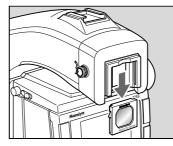
**2.** Remove the existing diopter by sliding downwards using the fingernail groove and detach.
