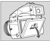
**2.** Remove the camera rear cap by putting a finger into the notch and sliding the cap down.
