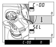
1. Turn on the power. Turn the shutter release mode lever to the "S" or "C" position.
