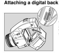
1. When detaching the digital back, pull back the detachment lever (found on the right side on ZD backs) or press the release button (found on the left side of M series backs) and pull away from the camera body.
