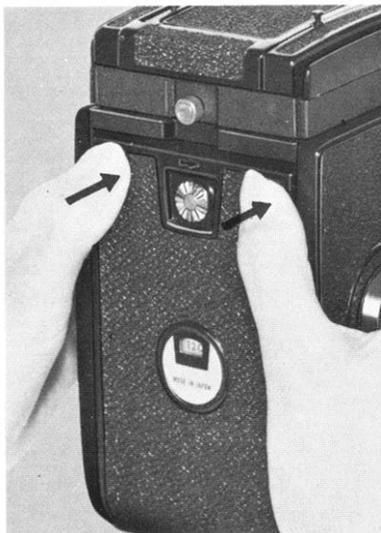
When closing the back cover, firmly press both sides of the back cover catch button, making sure that neither side of the back cover is open or loose. Unless the back cover is closed tightly, the automatic film stopper will not work. Also, if only one side of the back cover is pressed when closing, the automatic film stopper may not function.
