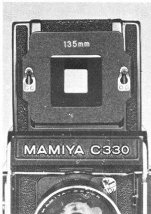
**3** When using the 105 mm, 135mm, 180mm, or 250mm lens, attach the respective sportsfinder mask for the lens used on the finder mask stud (11), adjusting for the change in field of view.
