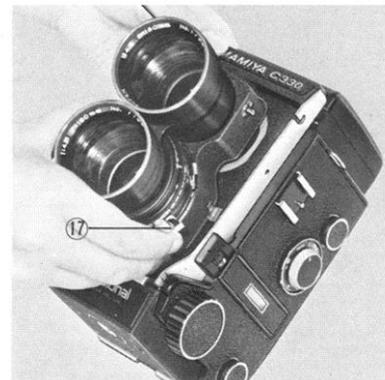
To attach another lens to the camera body, carefully position the lens so that the lens shutter cocking lever (17) connects with the cocking lever on the camera body. This operation is correctly performed by previously cocking the lens shutter with the fingers, first inserting the lens from the cocking lever side on the body. Clamp the lens catch (20) to its original position, and turn the lens change knob (24) clockwise to the "LOCK" position. With this operation, lens replacement is completed.
