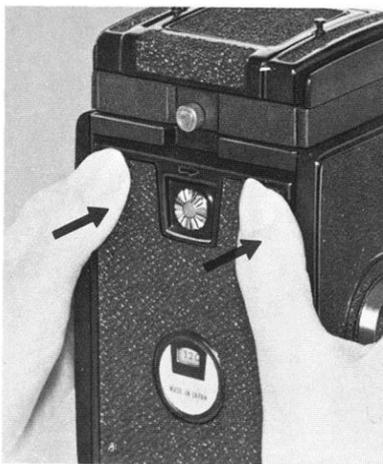
**3** Close the back cover. When closing the back cover, firmly press both sides of the back cover catch button. Twist the button counter-clockwise, so that the back cover does not open unexpectedly.
