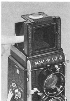
**5** To return the sportsfinder flap (12), push the magnifying glass, fold the side plates inward and the back plate downward, finally folding the finder frame (9).
