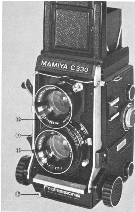
1. After focusing, turn the shutter speed ring (15) and set the shutter speed; then adjust the aperture of the lens by turning the aperture control knob (18). Now the camera is prepared for taking pictures.
