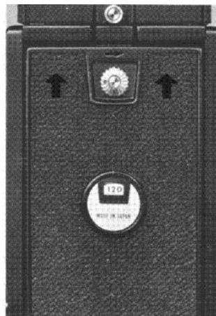
When closing the back cover, firmly press both sides of the back cover catch button.
