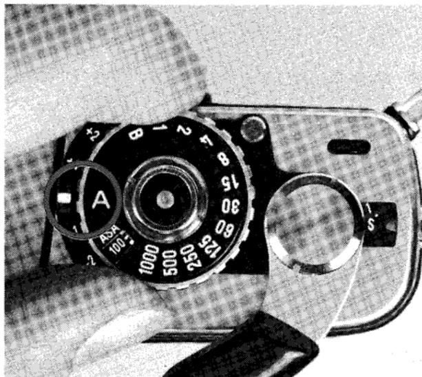
2. Set the desired lens opening by turning the aperture ring on the lens barrel. The shutter speed as indicated by lighted LED at the right of the frame will vary automatically to yield proper exposure for the aperture and other settings with the light being metered.
