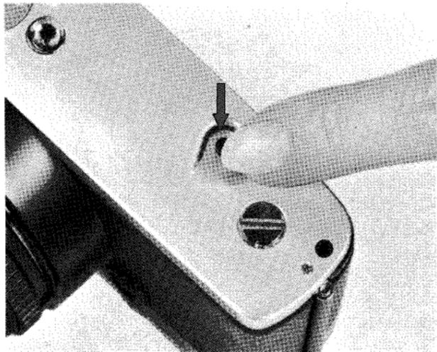
2. Unfold the rewind crank and turn it in the direction indicated by the arrow on it until the red Safe Load Signal bar moves out of the window to the left. You will then feel tension on the film increase and disappear, and the crank will turn freely.
