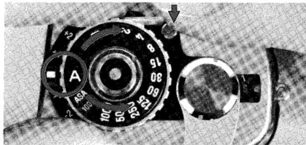
The shutter-speed/function selector will lock at normal automatic setting and there are click-stops at each half stop setting.
