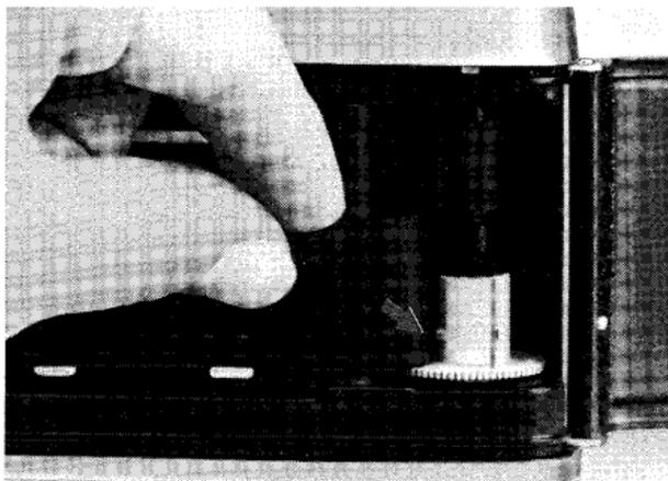
4. With the shutter speed function selector on manual setting operate the film-advance lever slowly until the film has begun to wind firmly around the take-up spool and the sprocket teeth are engaged with holes on both edges of the film. If the advance lever stops at the end of a full stroke during this procedure, release the shutter and continue.
