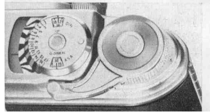
the illustration on page 8 shows the position of the needle at exposure value number 10. Frequently the needle (16) does not point to the centre of the field, but, as shown on the illustration on this page, points to an intermediate value. If the accuracy of the exposure value meter is to be fully used the intermediate exposure value — in this instance 9,5 — should be read.
