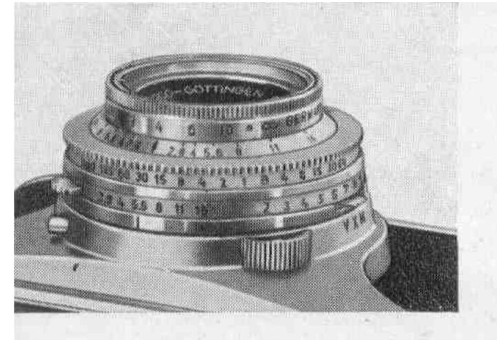
**Example:** At a distance of about 10 ft. (3 m.) selected at random and shown on the illustration, the depth of focus range extends:
