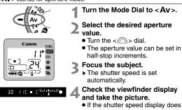
If the shutter speed display does not blink, a correct exposure will be obtained.
