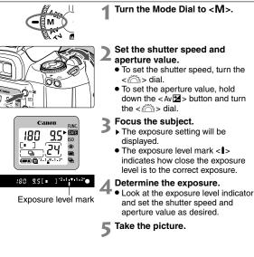
If the exposure level mark <1> blinks at the <2+> or <-2> level, it indicates that the difference between the standard exposure exceeds +/-2 stops.
