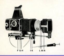
lens, viz: the lens remains at a fixed distance from the subject to be photographed. This means that the frontshade can be extended to provide the desired screening effect by loosening screw (1) and unclipping the hooks (N) on both sides of the frontshade. The frontshade also functions as a holder when carrying out reproduction work with Hasselblad Transparency copy holder (TIADC).
