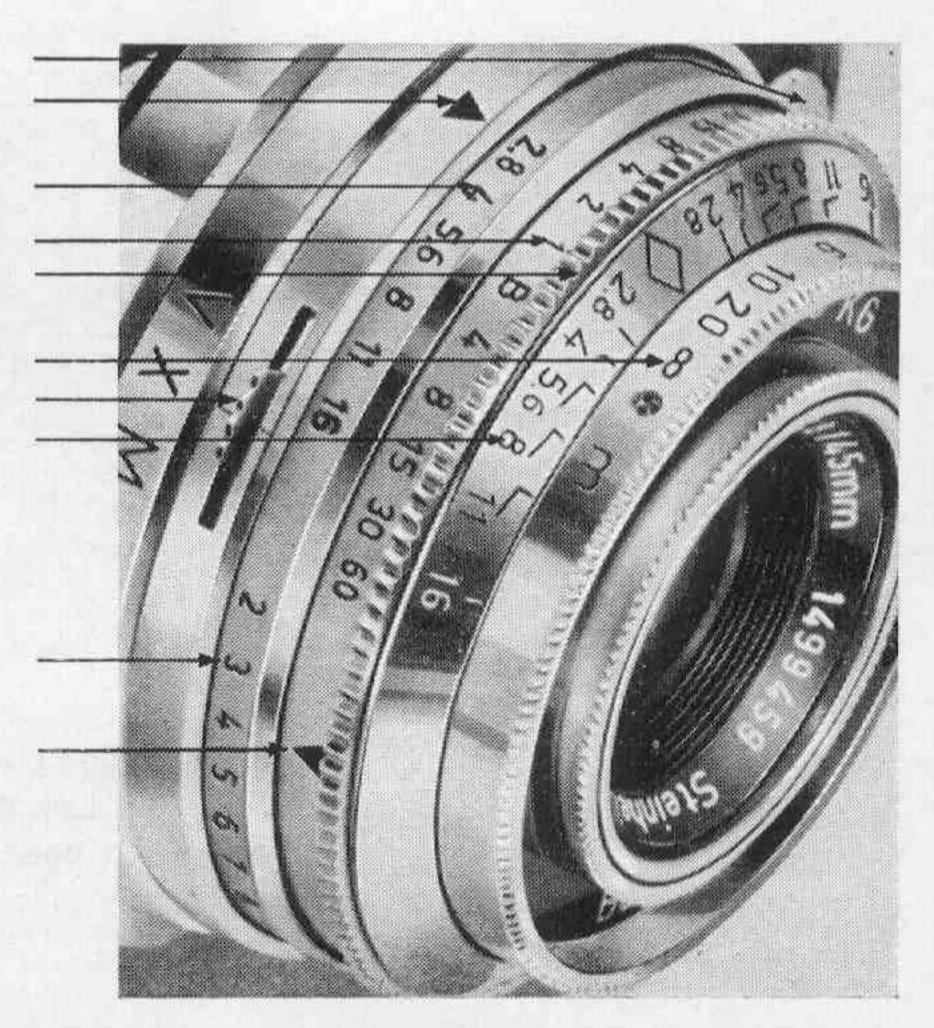
4. With the REGULA camera, this has been simplified for you, by providing a light value scale (LVS) exposure meter, built by the world's most famous and largest manufactures of exposure meters — Gossen. This meter provides a LV reading at which the shutter must be set. Hence at LV "10" you would be in a position to choose any combination of shutter speed and diaphragm, as illustrated above in para. 3. To do this, the following action is taken:
