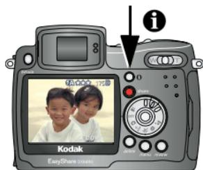
The icons that appear on the EVF or the LCD screen indicate the active camera and picture settings.
