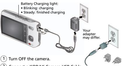
2 Connect a KODAK Camera USB Cable, Micro B / 5-Pin. (Use only the cable included with this camera!)
