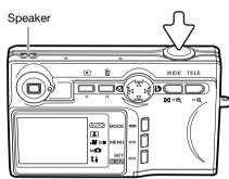
Press the shutter-release button to start the playback of the displayed file.
