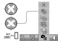
**Center-weighted metering:** measures luminance over the entire image area with emphasis to the central region. This metering mode give accurate exposures in almost all situations.
