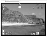
The operation of the program exposure mode is the same as described in the basic recording operation section on page 24. However, when the shutter-release button is pressed partway down, the shutter speed and aperture used for the exposure are displayed in the top right corner of the monitor.
