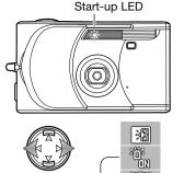
Use the left/right controller keys to select the monitor menu section.
