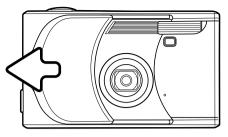
Slide the lens cover in the direction indicated to turn on the camera; the lens extends automatically. Do not touch or hinder the lens while it is extending.
