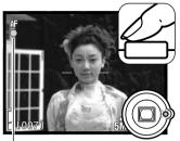
Place the subject within the AF area. Press and hold the shutterrelease button partway down and wait until the focus signal appears and viewfinder indicator lamp glows to indicate focus is locked. If the signal and lamp blink, repeat the procedure.
