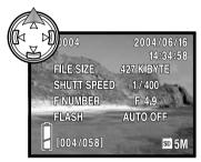
Press the up key of the controller to display image information. Press the up key a second time to hide the information display.
