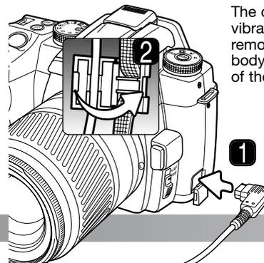
The cord can be attached to the camera strap. Open the remote-cord clip on the strap and push the cord into the groove. Close the clip until it clicks into place (2).
