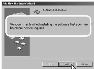
The last window confirms the driver has been installed. Click “Finish” to close the add new hardware wizard. Restart the computer.
