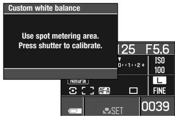
A guidance message appears. If the shutter-release button is pressed partway down, the monitor display returns. The red custom set indicator is displayed in the white-balance panel. Turn the white-balance dial to another position to cancel the routine.
