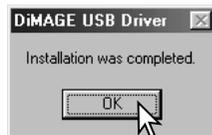
When the driver has been successfully installed, a window appears. Click "OK." Restart the computer before connecting the camera (p. 115).
