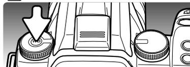
With the white balance dial in the preset white balance position, press the white-balance button to open the setting screen.
