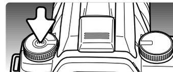
White balance can be set to a known color temperature of a light source or set to the color temperature determined by a color meter. With the white balance dial in the color temperature (K) position, press the white-balance button to open the setting screen.
