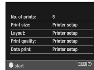
Once printing begins, the operation can be canceled by pressing the center of the controller. The printing-finished message indicates the end of the operation; press the center of the controller and turn the camera off to end the routine.
