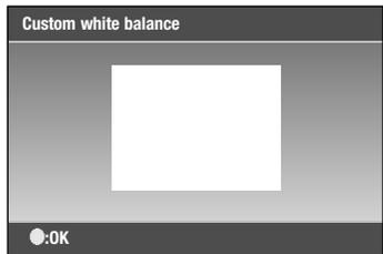
An image of the reference target is displayed. Press the central button of the controller to complete the operation.
