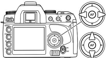
Use the left/right keys of the controller to highlight the appropriate menu tab; the menus change as the tabs are highlighted.
