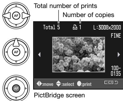
The number of prints in the print run are displayed as well as the print parameters selected with the menu. See the menu navigation section for more information (p. 128). Press the central button of the controller to begin printing, or press the menu button to return to the PictBridge screen.
