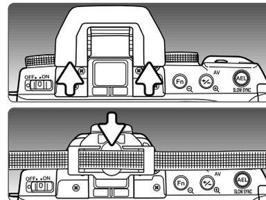
Carefully slide the eyepiece cup from around the viewfinder frame by pushing on each side of the cup.
