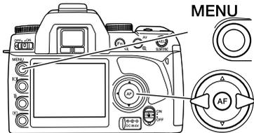
Activate the recording menu with the menu button. Tab 1 at the top of the menu is highlighted.
