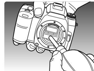
Turn the camera off to complete the operation. Replace the lens or body cap.
