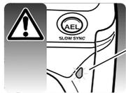
Never disconnect the camera when the access lamp is lit - the data or memory card may permanently be damaged.
