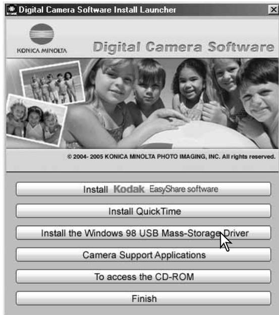
Before connecting the camera to the computer, place the Digital Camera Software CD-ROM in the CD-ROM drive. The Digital Camera Software installer launcher opens. To automatically install the Windows 98 USB driver, click on the "Install the Windows 98 USB mass-storage driver" button. A window appears to confirm that the driver should be installed; click "Yes" to continue.
