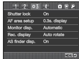
To lock the shutter when no lens is mounted (p. 97).
