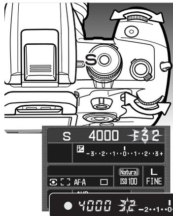
Shutter priority is set with the exposure-mode dial (p. 39). The photographer selects the shutter speed and the camera sets the appropriate aperture to ensure correct exposure.
