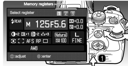
To save the current camera settings, press the M SET button (1); the setting appear on the registration screen.
