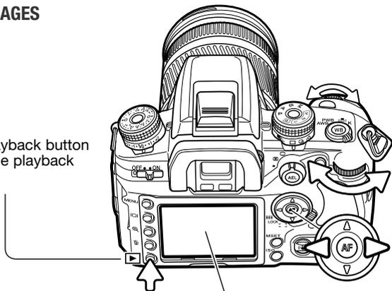
The left/right keys of the controller and both control dials can be used to scrolls through the images.
