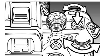
The control dials and the left/right controller keys select a previous custom setting stored on register 1, 2, or 3, or the set option to calibrate the camera.
