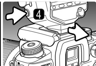
1. Remove the accessory shoe cap (p. 117) and slide a Program 5600HS(D) or 3600HS(D) flash on the accessory shoe until the safety lock engages.
