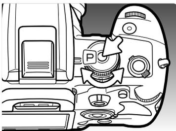
Full-auto program is set with the exposure-mode dial. Use this exposure mode when wanting fully automatic operation.
