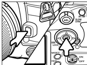
Simultaneously press and hold the lens release and the central button of the controller.
