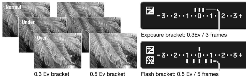
To make a flash bracket, raise the camera flash; the ambient exposure is not bracketed. The flash recharges between exposures. Exposure brackets are made when the flash is down.
