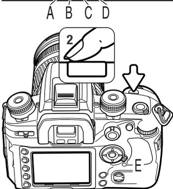
Press the shutter-release button all the way down (2) to take the picture. Press the shutter-release button gently so as not to shake the camera during the exposure.
