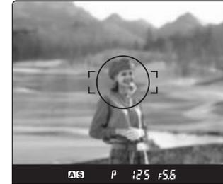
2. Half-press the shutter release button, and focus will be adjusted automatically.
