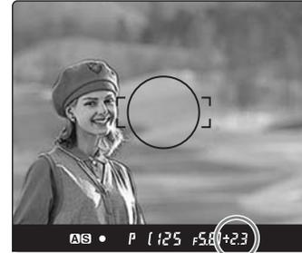
Keep pressing the AEL button **A**, and the difference between the metered exposure value and the exposure of the new composition will be displayed on the viewfinder LCD. This function can be used to see if an object of very different brightness levels can be properly captured.
