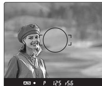
★ When the focus mode is set at “S” (single focus mode) and the ● focus mark is lit, hold the shutter release button halfway down to lock the focus.
