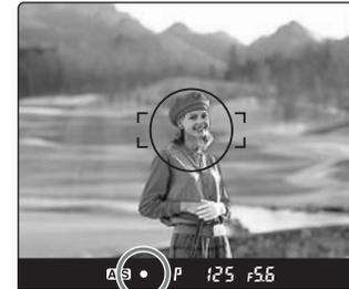
When the focus mark ● lights, the picture is in focus.
