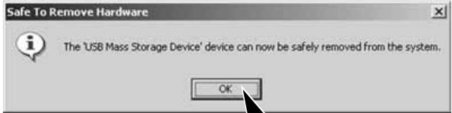
When more than one external device are connected to the computer, the unplug-or-eject-hardware window can be used. To disconnect the camera, double click on the unplug-or-eject-hardware icon located on the task bar to activate the window.
