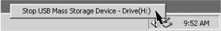
Click on the small window to stop the device. The safe-to-remove-hardware window will appear. Click "OK." Turn the mode dial to another position and then disconnect the USB cable.
