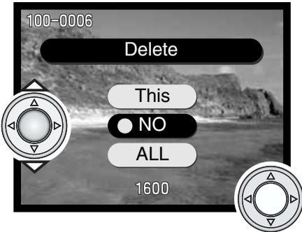
Use the up/down controller key to highlight the delete option. Press the controller to execute the command.
