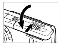
6 Fold the battery/card-chamber door down and slide it slightly toward the front of the camera. Then, while using a downward pressure, slide it back to the rear of the camera until it clicks.
