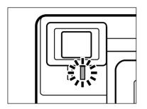
When the shutter-release button is pressed part-way down, the autofocus system locks focus at the subject distance. The focus lamp (green) will indicate the focus status when the shutter-release button is pressed part-way down.
