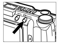
Press the display/ENTER button to turn on the LCD monitor if desired.
