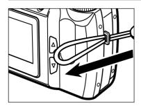
Insert the smaller loop of the strap through the strap eyelet.
