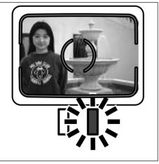
Without lifting your finger, recompose the picture, then press the shutterrelease button all-the-way down to take the picture.
