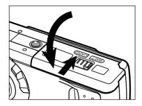
Fold the battery/card-chamber door down and slide it slightly toward the front of the camera. Then, while using a downward pressure, slide it back to the rear of the camera until it clicks.
