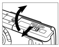
2 Open the battery/card-chamber door by sliding it in the direction indicated, then open the door.
