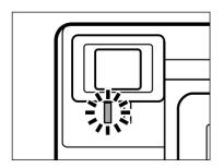
The orange flash lamp will indicate the flash status when the shutter-release button is pressed partway down.
