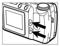
2 Press the ▲ or ▼ button until the desired indicator is displayed in the data panel.  When you press the ▲ button, the flash modes will change as follows:
