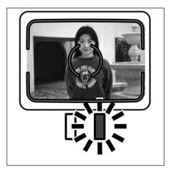
1 Place the focus frame on your subject or center the subject in the LCD monitor, then press and hold the shutter-release button partway down so the green focus lamp glows.
