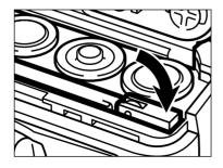
3 Fold the card-release lever down as shown.
