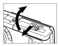
Open the battery/card-chamber door by sliding it in the direction indicated, then open the door.
