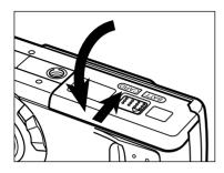
4 Fold the battery/card-chamber door down and slide it slightly toward the front of the camera. Then, while using a downward pressure, slide it back to the rear of the camera until it clicks.
