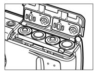
Insert the batteries as indicated by the +/- diagram on the back of the battery/card-chamber door.
