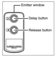
Point the emitter window toward the remote-control receiver on the front of the camera.
