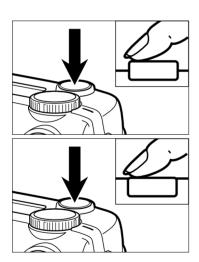
7 Press the shutter-release button partway down.
