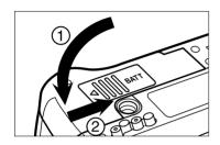
4 Close the battery-chamber door in the direction of the arrow (1) and slide it until it clicks (2).
