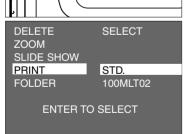
2 Press the ▲ or ▼ key so that [PRINT] is highlighted and press ▶ key.
