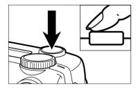
7 Press the shutter-release button partway down.
