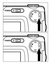
1 In the recording mode, press the ► key in the recording mode so that the image is zoomed to the maximum.
