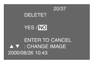
\* The colour of the background in the left figure is gray so that you can easily find out the contents of the display. However, the image to be deleted (the image displayed on the LCD monitor in step [1]) is actually displayed in the background.
