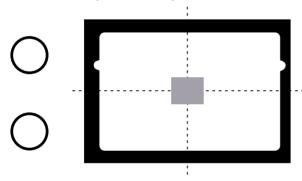
In the autofocus mode, the focus is adjusted at the gray part as shown in the figure.
