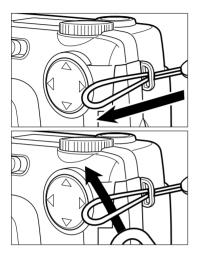
1 Insert the smaller loop of the hand strap through the strap eyelet.
