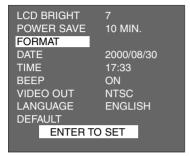
3 Press the ▲ or ▼ key so that [FOR-MAT] is highlighted and press the ENTER button.
