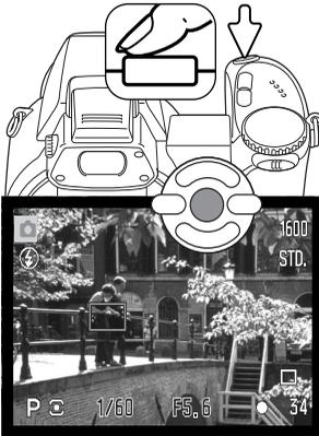
Take the picture as described in the basic recording section; press the shutter-release button partway down to lock focus and exposure. Press the shutter-release button all the way down to take the picture.
