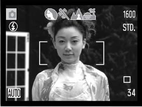
A row of gray indicators at the top on the monitor display will indicate Automatic Digital Subject Selection is active. Place the subject in the focus frames; the procedure is the same as the basic recording operation described on page 22.
