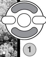
Use the up/down keys of the controller (1) to set the aperture. The aperture value can be changed in 1/3 stop increments. Press the shutter-release button partway down to activate the exposure system; the corresponding shutter speed will be displayed on the monitor.
