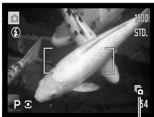
The drive modes control the rate and method images are captured. The drive mode is set on all menus except the movie menu. With auto recording and Digital Subject Programs, the drive mode is reset to single-frame advance when the exposure-mode dial is moved to another position or the camera is turned off. In P, A, S, and M exposure modes, the drive mode remains in effect until changed. Refer to the following sections for descriptions of the drive modes.
