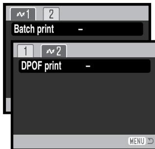
After the batch-print option is chosen, the USB DIRECT-PRINT selection screen will show which images and the number of copies selected. The controller can be used to edit the print order, see page 102.
