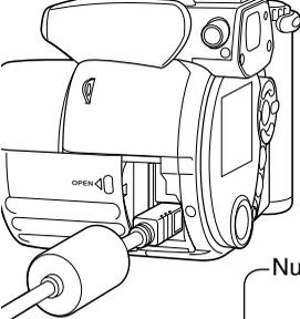
Connect the camera to the printer using the camera's USB cable. The larger plug on the cable is connected to the printer. Open the card chamber door and insert the smaller plug of the cable into the camera. Turn the camera on; the USB Direct Print screen is displayed automatically.
