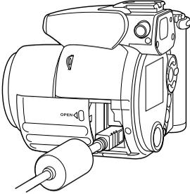
Connect the camera to the printer using the camera's USB cable. The larger plug on the cable is connected to the printer. Open the card chamber door and insert the smaller plug of the cable into the camera.
