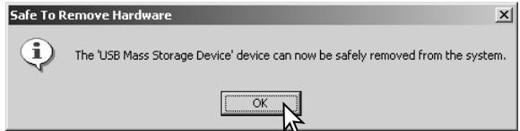
When more than one external device are connected to the computer, repeat the procedure above except right click on the unplug-or-eject-hardware icon. This will open the unplug-or-eject-hardware window after clicking on the small window indicating the unplug-or-eject-hardware routine.
