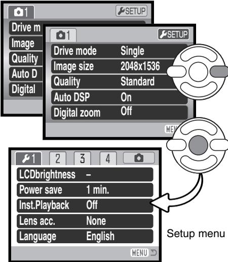
Use the right key of the controller to highlight "setup" at the top of the menu.
