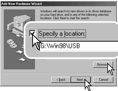
Choose to specify the location of the driver. The browse window can be used to indicate the driver location. The driver should be located in the CD-ROM drive at :Win98\USB. When the location is shown in the window, click “Next.”
