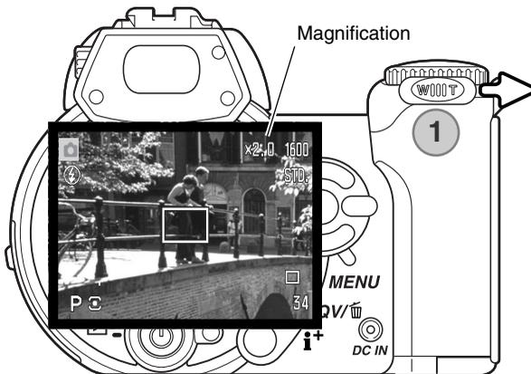
The digital zoom is operated by the zoom lever (1). Slide the lever right (T) to zoom in to the telephoto position of the lens. When the digital zoom activates, the image magnification will be displayed on the monitor. Turn the lever left (W) to zoom out.
