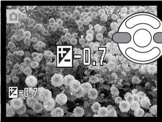
To adjust the exposure, press the left or right controller key; the exposure-compensation screen appears.
