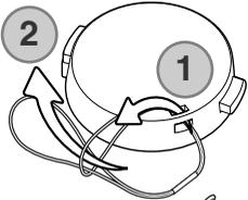
Pass one of the small loops of the lens-cap strap through the eyelet on the lens cap (1). Pass the other loop through the first loop and tighten (2).
