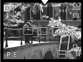
Use the left/right keys of the controller to highlight the desired autofocus area; the active area is blue.
