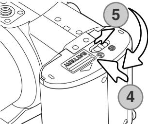
Close the battery-chamber door and slide it toward the body (4) to engage the safety catch. Slide the battery-chamber lock to the close position (5).
