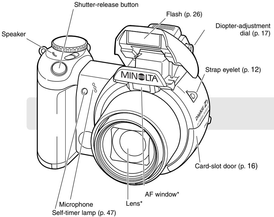
The USB port and AV-out terminal are located behind the card-slot door. The battery-chamber door (p. 13) and tripod socket are located on the bottom of the body.
