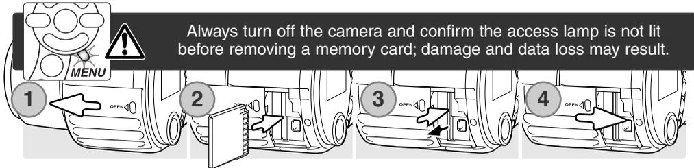
1. Open the card-slot door by sliding the door toward the front of the camera.
