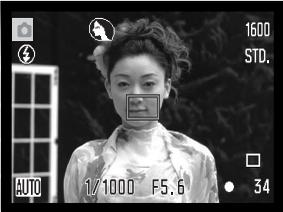
Press the shutter-release button partway down; the AF system will locate the subject and the Automatic Digital Subject Selection function will choose a subject program. If no indicators are displayed, programmed AE is active. Press the shutter-release button all the way down to take the picture. Hold the camera steadily when the sunset subject program is selected as exposures can be long.
