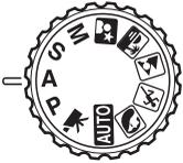
The photographer selects the aperture and the camera sets the appropriate shutter speed to ensure the correct exposure. When aperture priority is selected, the aperture value on the monitor turns blue and a double arrow indicator appears next to it. The flash mode can be set to fill-flash, fill-flash with red-eye reduction, or slow sync. (p. 26).
