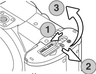
To open the battery-chamber door, slide the lock to the open position (1). Slide the door the the side of the camera (2) to release the safety catch. Lift the door to open (3).
