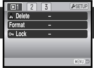
Single, multiple, or all files on the memory card can be deleted in section 1 of the playback menu (p. 70). The delete option has three settings:
