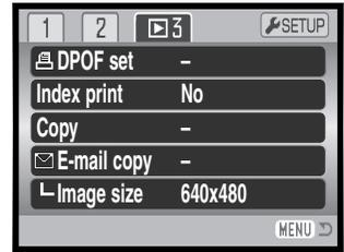
When a copy function is used, a folder is created for the files (p. 98); copy files are placed in a folder with a name ending in CP, and E-mail Copy images are placed in a folder ending in EM. The same folder is used to store copies until the number of images exceed 9,999. Copies of locked images are unlocked. DPOF information is not copied.
