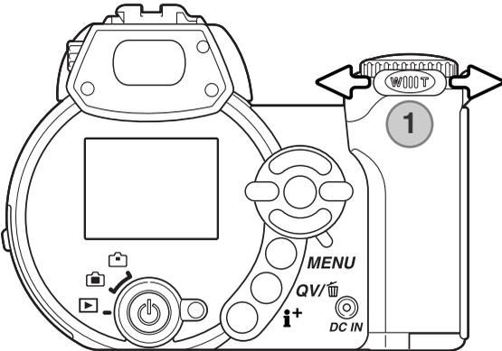
The zoom lever controls the lens (1). Sliding the lever to the right (T) will zoom in to the telephoto position of the lens. Sliding the lever to the left (W) will zoom out to the wide-angle position.
