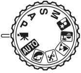
This camera can record digital video with sound. Total recording time varies with the image size and frame rate, see page 66. Exposure compensation and the macro modes can be used. Other changes can be made with the movie recording menu (p. 44).
