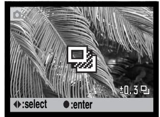
When selecting custom white balance, the calibration screen appears. Fill the frame with a white object and press the central button of the controller to calibrate the camera.
