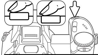
Frame the picture as described in the basic recording operation section (p. 22). Press the shutter-release button partway down to set the the focus and exposure. Press the shutter-release button all the way down and release to start recording.
