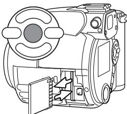
When the change-card message is highlighted, remove the camera's memory card and insert the card to which the image should be copied. Press the central button of the controller to continue or the menu button to cancel the copy operation.
