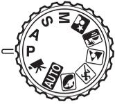
The program exposure mode controls both the shutter speed and aperture to ensure correct exposures. This exposure mode allows photographers to shoot without worry about exposure settings. The shutter speed and aperture values of the exposure are displayed on the monitor when the shutter-release button is pressed partway down. If shutter speed and aperture displays turn red, the scene is beyond the exposure control range of the camera.
