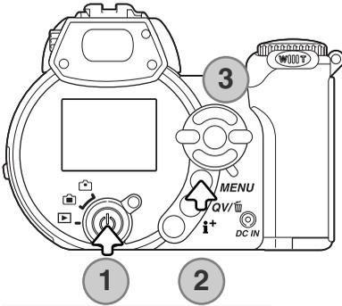
Press the main switch (1) to turn the camera on. Press the menu button (2) to open the menu; the appearance of the menu will depend on the position of the camera's controls.
