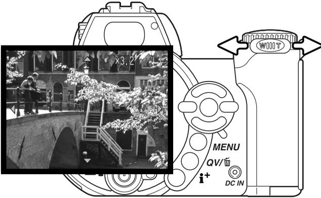
With the image to be magnified displayed, slide the zoom lever to the right (T) to activate the enlarged playback mode. The degree of magnification is displayed on the LCD monitor.
