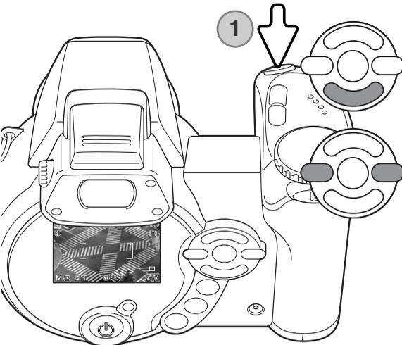
Use the down key of the controller to decrease the shutter speed below 15 seconds until "T" is displayed.
