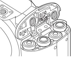
Insert the batteries as indicated on the diagram on the inside of the battery-chamber door. Confirm the positive and negative battery terminals are oriented correctly.
