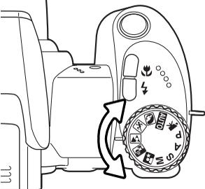
Digital subject programs optimize the camera's exposure, white-balance, and image-processing systems for specific conditions and subjects. Simply turn the exposure mode dial to select the appropriate subject program; the active subject program is displayed in the bottom left corner of the monitor
