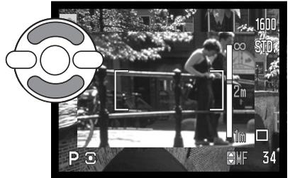
When using the shutter-priority, aperture-priority, or manual exposure modes (p. 36 - 38) with manual focus, press the central button of the controller to switch between using the up/down keys to focus or to adjust the exposure. The active function is indicated in blue.
