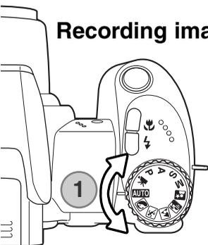
Turn the exposure-mode dial to the auto-recording position (1); all camera operations are now fully automatic. The autofocus, exposure, and imaging systems will work together to bring beautiful results effortlessly.
