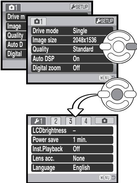
Use the right key of the controller to highlight setup tab at the top of the menu.
