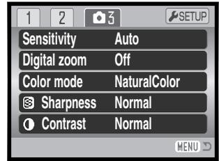
The auto setting automatically adjusts the camera sensitivity to the light conditions between ISO 50 and 200. When any other setting than auto is used, "ISO" and the set value will be displayed on the monitor.
