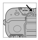
2. Turn the camera upside-down, then press the film-chamber release to open the film chamber.
