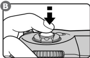
The camera will adjust focus automatically, and the results of the autofocus operation will be displayed in the viewfinder.
