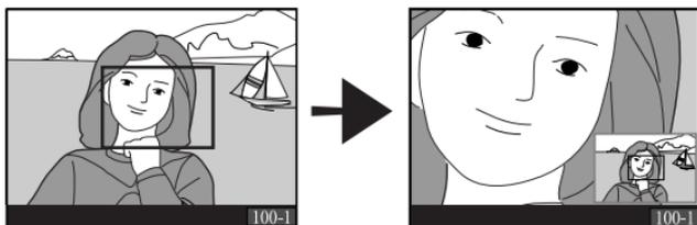
The center of the image will be enlarged to fill the monitor. To view other areas of the photograph, press the multi selector. To cancel zoom and return to normal playback, press the **FUNC** button.
