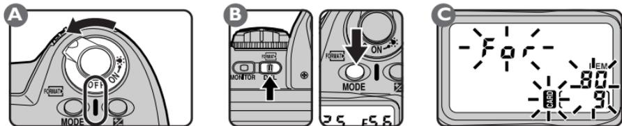
When formatting is complete, the frame-number display in the control panel on top of the camera will show **1**, and the maximum number of shots that can be stored on the card at current settings will be shown in both control panels (if more than a hundred exposures can be stored on the card, the display will show **FL**).
