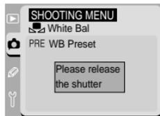
**4** Under the lighting that will be used in the actual photograph, frame a white or neutral gray object so that it fills the viewfinder and then press the shutter-release button all the way down. The shutter will be released and the measured value for white balance stored in camera memory, but no image will be recorded to the memory card.
