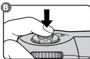
When focus is locked by pressing the shutter-release button halfway, you can take several photographs in succession at the same focus setting by keeping the shutter-release button lightly pressed between each shot. Focus will also remain locked between shots as long as you continue to press the AE-L/AF-L button.
