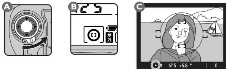
The focus area can be fixed at the chosen setting by rotating the multi selector lock to the locked position.
