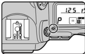
To use TTL flash control, connect an SB-28DX or SB-50DX Speedlight to the camera and set the flash to D-TTL auto-flash mode. Depending on the type of lens used, one or more of the following TTL flash modes will be available. TTL flash control is available only with the SB-28DX and the SB-50DX.
