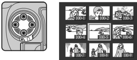
To scroll through thumbnails a page at a time, press the
