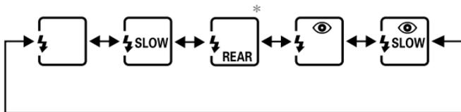
\* In programmed auto and aperture-priority auto modes, the mode icon shown at right will be displayed when the flash mode button is released.
