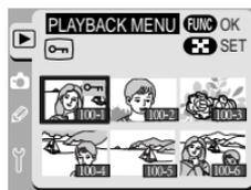
To protect an image, highlight it and press the **FUNC** button. The image will be marked with a **LOCK** icon (to deselect an image, highlight it and press the **FUNC** button a second time). Repeat until all the images you wish to protect have been selected, then press the **MENU** button to put any changes into effect and exit the thumbnail menu.
