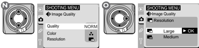
Repeat C–D to display the Image Quality menu, then highlight **Resolution** (N) and press the multi selector to the right to display the Resolution menu (O).
