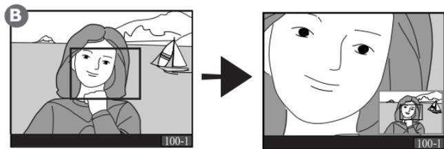
For approximately two seconds after you press the **FUNC** button to zoom in on the image, or after you press the multi selector to scroll the image, a thumbnail showing your current position in the image will appear in the bottom right corner of the display.
