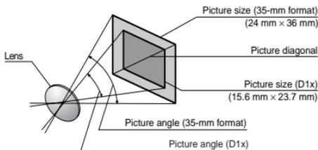
The diagonal picture angle of a 35-mm camera is roughly 1.5 times that of the D1x. Consequently when a lens of a given focal length is attached to the D1x, the corresponding focal length in 35mm format at the D1x's picture angle can be calculated by multiplying the focal length of the lens by 1.5. The following chart shows some examples:
