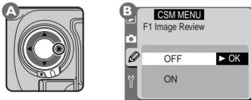
Press the multi selector up or down to highlight the desired option, then press the selector to the right to put your choice into effect and return to the custom settings menu. To return to the custom settings menu without changing settings, press the multi selector to the left.
