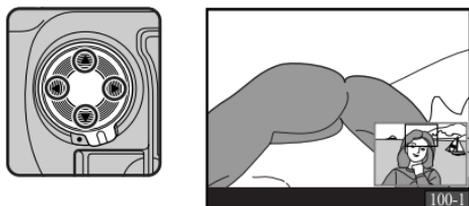
For approximately two seconds after you press the **FUNC** button to zoom in on the image, or after you press the multi selector to scroll the image, a thumbnail showing your current position in the image will appear in the bottom right corner of the display.
