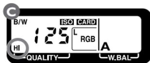
As the main command dial is rotated, settings will change in the order shown below (an image quality of JPEG Normal appears in the rear control panel as **NORM**).
