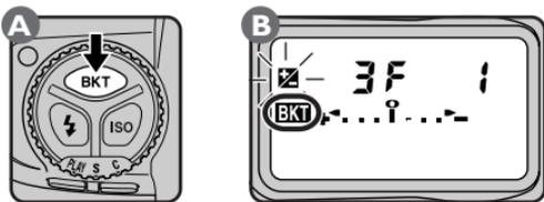
2 Pressing the BKT button (A), rotate the sub-command dial (B) to choose a bracketing program (C).
