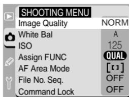
Press the **MENU** button to display the camera menus (A), then unlock the multi-selector and press it up or down until the shooting menu is displayed (B). Press the multi-selector to the right to enter the shooting menu (C).
