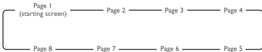
Page 6 (image histogram) and Page 7 (image highlights) are only shown if the appropriate option has been selected in the **Display Mode** sub-menu of the playback menu. Page 5 is only shown if a GPS unit was connected when the photograph was taken. Depending on the lens used, some information may not be displayed.
