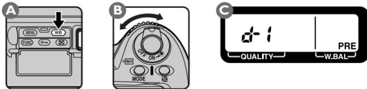
A setting of **d-1** is equivalent to Preset-1, **d-2** to Preset-2, and **d-3** to Preset-3.
