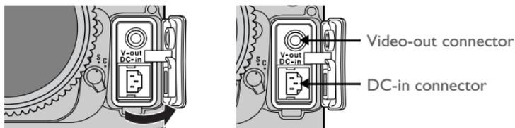
Connect the camera to the video device as shown below.
