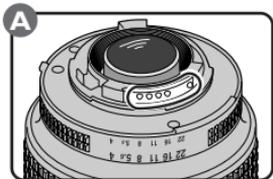
Nikkor lens with built-in CPU (CPU lens)
