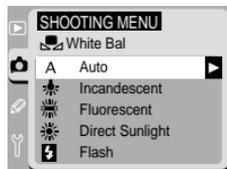
Except in the case of **WB Preset** (preset white balance), highlighting a white balance setting and pressing the multi selector to the right displays a dialog where you can fine-tune the chosen setting. Press the multi selector up or down to choose the amount white balance will be adjusted, then press the multi selector to the right to put your selection into effect and return to the shooting menu.
