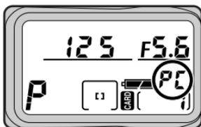
If the mode dial is set to PC and the camera is not connected to a computer, or if it is connected when neither Nikon View 4 nor Nikon Capture 2 is running, the camera will function as in single-frame or continuous mode, the only difference being that the shooting mode (single-frame or continuous) is selected using Custom Setting 30 (**PC Shooting Mode**).
