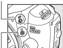
**Fn (☺) button:** release mode, image quality and size, ISO sensitivity, white balance, Active D-Lighting, or bracketing
