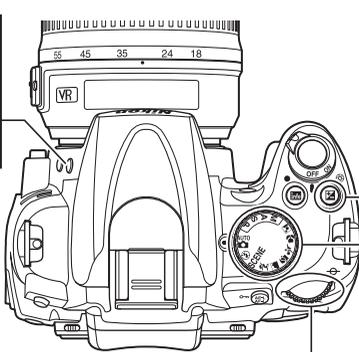
**☑ button:** aperture, exposure compensation, and flash compensation
