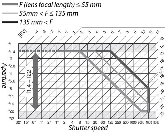
The maximum and minimum values for EV vary with ISO sensitivity; the above graph assumes an ISO sensitivity of ISO 200 equivalent. When matrix metering is used, values over  $17\frac{1}{3}$  EV are reduced to  $17\frac{1}{3}$  EV.
