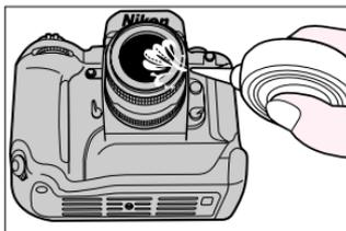
5. Clean lens surface with a blower brush. To remove dirt and smudges, use a soft, clean cotton cloth or lens tissue moistened with ethanol (alcohol) or lens cleaner. Wipe in a circular motion from center to outer edge, taking care not to leave traces and not to touch the other lens parts.
