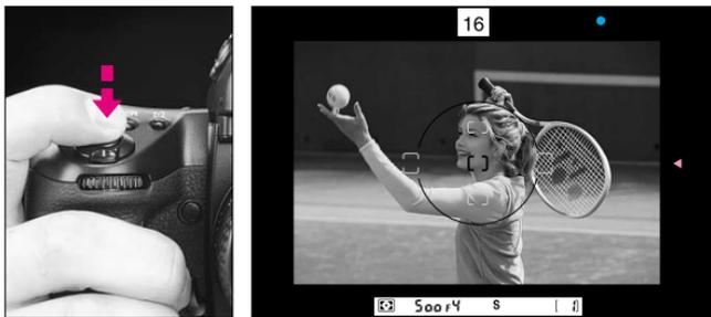
**3** Look inside viewfinder, compose and lightly press shutter release button. Confirm the automatically set aperture value.
