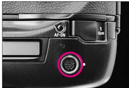
A 10-pin remote terminal is provided for remote operation of the F5 with Personal Computer Connecting Cord MC-33 or MC-34, Remote Cord MC-20 or MC-30, etc. For available remote control accessories, see page 145.
