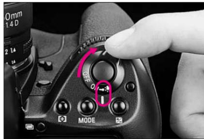
In dim light, rotate Power/LCD panel illumination switch toward
