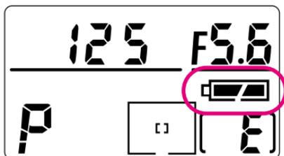
Rotate power switch to **ON** position while pressing the lock release, and confirm that the full battery mark appears in the top LCD panel, indicating sufficient battery power. The battery mark and exposure indications automatically turn off after 8 sec.
