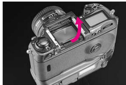
2 Insert your fingernail under the rear edge of the screen and lift the focusing screen out.
