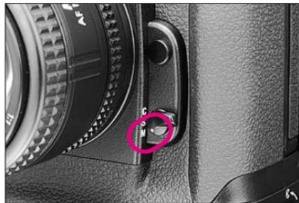
To focus manually when using Nikon lenses that do not have an A/M switch, set the camera's focus mode selector to M. When using a Nikon lens that has an A/M switch, set the lens' switch to M; when using an AF-S or AF-I Nikkor lens, set the switch to M or M/A; with these lens types it is not necessary to change the camera's focus mode selector.
