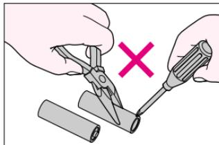
2. **Do not** disassemble, short circuit or heat batteries. **Do not** charge dry cells.
