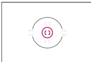
4 Select Single Area AF mode by rotating the Main-Command Dial while pressing the AF area mode (AF) button.
