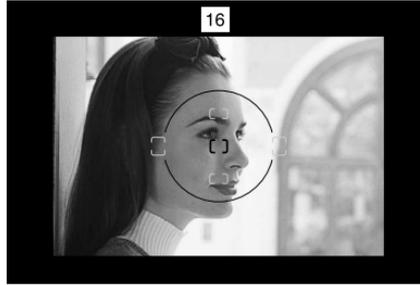
**1** Center main subject inside viewfinder and/or move in closer until the reference circle for Center-Weighted Metering or Spot Metering is fully covered by the subject.
