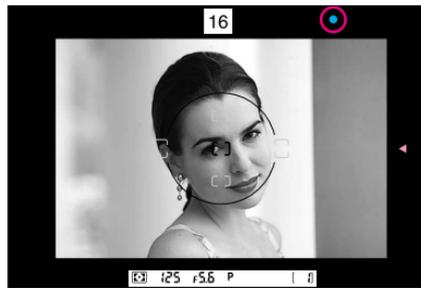
Lightly press shutter release button to start autofocus operation. When the subject is in focus, the camera's autofocus motor (or the built-in motor of an AF-S or AF-I Nikkor lens) stops driving the autofocus lens and ● appears in the viewfinder. Unless you remove your finger from the shutter release button, the motor will start driving the lens again to obtain an in-focus picture if the focus distance changes.
