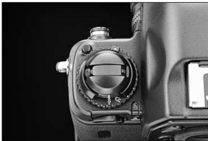
There are four automatic film advance modes. To choose a mode, rotate the film advance mode/self-timer selector while pressing the film advance mode selector lock release. Set **S** for Single-frame shooting, **CL** for Continuous low-speed shooting, **CH** for Continuous high-speed shooting or **Cs** for Continuous silent-low-speed shooting.
