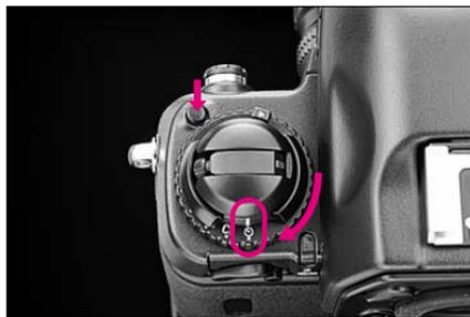
1 While pressing the lock release, set the film advance mode/self-timer selector to
