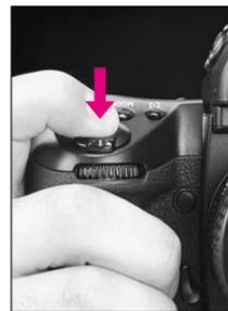
3 Confirm in-focus indicator ● appears, then fully depress shutter release button to take the picture.
