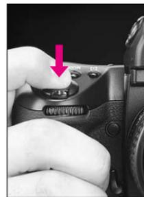
**3** While holding AE-L/AF-L button in, recompose, then fully depress shutter release button to take picture.
