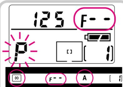
**If you are using a lens without CPU, or accessories such as bellows or extension rings**
