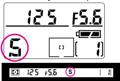
1 While pressing **MODE** button, rotate Main-Command Dial until **S** appears in the top LCD panel and **S** in the viewfinder.
