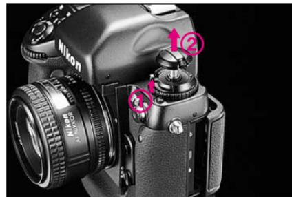
**13** Open camera back and remove film cartridge.
