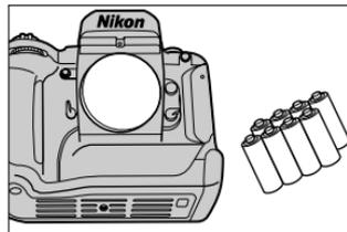
3. If you do not intend to use the camera for a long time, remove the batteries.
