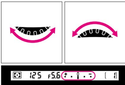
**3** Adjust shutter speed and aperture by rotating the Main- and/or Sub-Command Dials until the electronic analog exposure display shows desired exposure.
