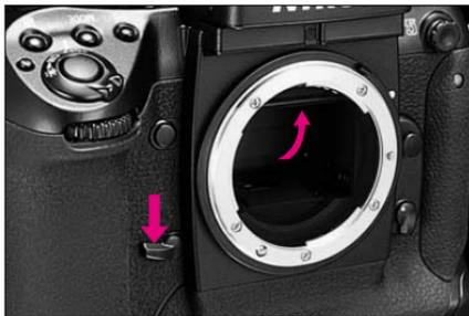
When using super-telephoto lenses or performing photomicrography, it is necessary to reduce camera vibration to the absolute minimum. Lock the reflex viewing mirror in the “up” position by rotating the mirror lockup lever counterclockwise until it stops.
