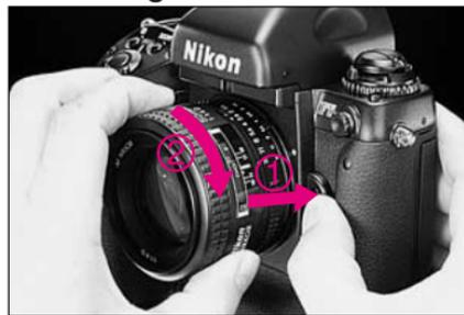
Push and hold lens release button and turn lens clockwise.
