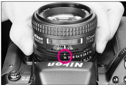
1 Make sure that the lens' aperture is set to its minimum position when using CPU Nikkor lens other than G-type.
