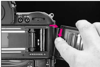
**2** Remove the camera back while pressing the camera back lock release.
