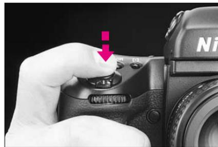
2 Compose picture, lightly press shutter release button, and confirm focus and exposure.
