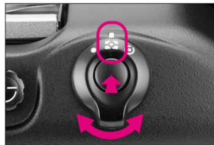
5 While pressing lock release, set the metering system selector to
