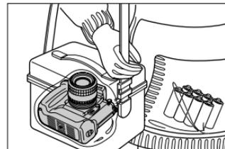
4. Battery power diminishes at extremely low temperatures — make sure the batteries you buy are new, and wrap the camera body in something warm.
