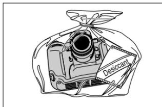
**11.** Store the camera in a cool, dry place away from naphthalene or camphor (moth repellent). In a humid environment, store the camera inside a vinyl bag with a desiccant to keep out dust, moisture and salt. Note, however, that storing leather cases in vinyl bags may cause the leather to deteriorate.
