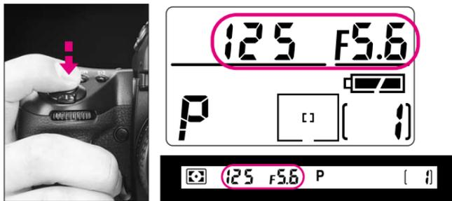
1 Make sure Programmed Auto exposure mode (P) is selected, and lightly press the shutter release button. Shutter speed and aperture appear in the top LCD and viewfinder.
