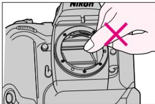
1. **Do not** touch the camera's reflex mirror or focusing screen. Remove dust with a blower brush.
