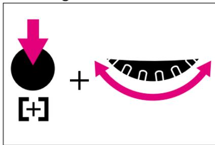
While pressing AF area mode (AF-ON) button, rotate the Main-Command Dial to select Single Area AF or Dynamic AF mode.
