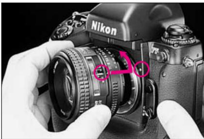
2 Position lens in the camera's bayonet mount so that the mounting indexes on lens and camera body are aligned. Taking care not to press the lens release button, twist lens counterclockwise until it locks into place.
