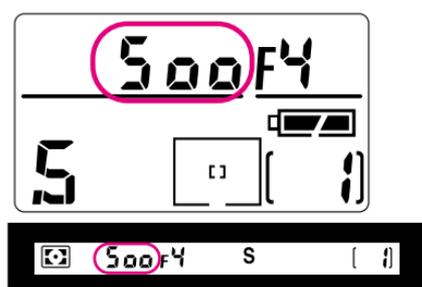
2 Remove finger from **MODE** button, and rotate Main-Command Dial to select desired shutter speed. Shutter speed indications change in 1/3 steps between 30 sec. and 1/8000 sec., and flash sync speed of 1/250 sec. (**x250**).
