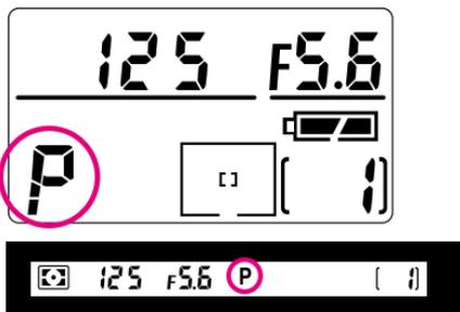
6 Select Programmed Auto exposure mode by rotating the Main-Command Dial while pressing the exposure mode (MODE) button so **P** appears in the top LCD panel and **P** in the viewfinder.
