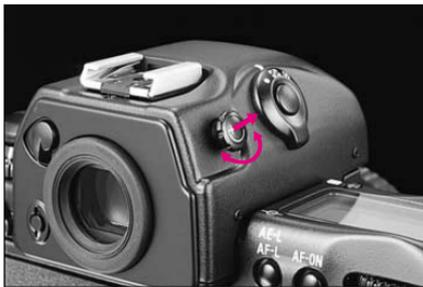
With supplied Multi-Meter Finder DP-30, adjusting the finder diopter enables near- or far-sighted photographers to adjust the eyepiece diopter within a continuous range of from  $-3$  to  $+1$ . Pull the diopter adjustment knob and rotate it in either direction until the focused image in 12mm-dia. circle within the viewfinder appears sharp, then push back to lock.
