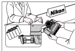
7. If the battery chamber is contaminated by battery leakage, take the camera to an authorized Nikon dealer.
