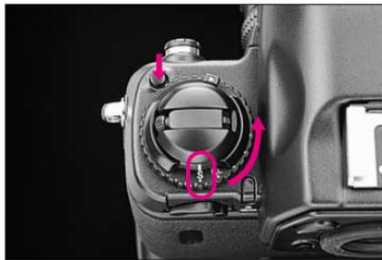
With the film advance mode at **S**, fully depressing the shutter release button takes one picture and automatically advances the film by one frame. Film advances immediately after the shutter closes whether you remove your finger from the shutter release button or keep the button depressed. To take the next shot, lift your finger from the button, then fully depress it again. Use Single-frame shooting for stationary subjects or subjects that do not require several frames of rapid firing.
