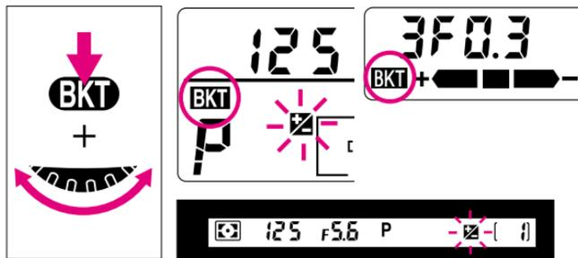
1 Rotate Main-Command Dial while pressing the **BKT** (Auto Exposure/Flash Exposure Bracketing) button to select Auto Exposure/Flash Exposure Bracketing mode. **BKT** appears in the top and rear LCD panels and
