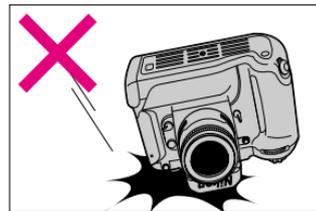
**9.** Make sure not to drop or bump the camera body/lens against a hard surface. Strong shock may cause malfunction.
