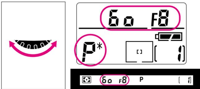
2 Rotate Main-Command Dial until desired shutter speed or aperture value appears in the viewfinder and top LCD panel. The Flexible Program indicator (**P\***) appears to indicate the program has been shifted or changed.
