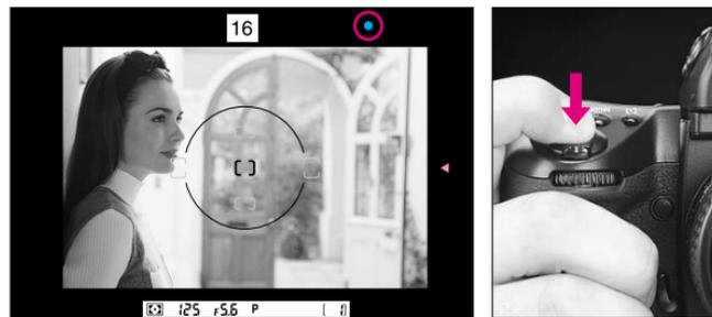
3 Keeping shutter release button lightly pressed, recompose, then fully depress shutter release button to take the picture.
