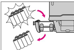
5. When replacing batteries, be sure to replace **all** batteries at the same time. Always use fresh batteries of the **same** brand.
