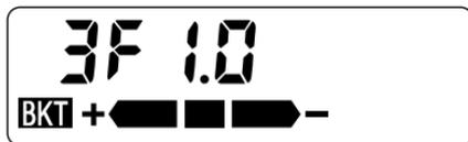
2 While pressing the **BKT** button, rotate Sub-Command Dial to select your desired number of shots and compensation value from one of the following:
