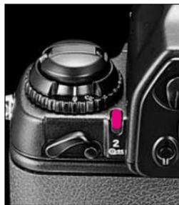
**10** At the end of the film roll, **End** blinks in the top LCD panel and viewfinder, the alert LED lights, and the shutter can no longer be released.
