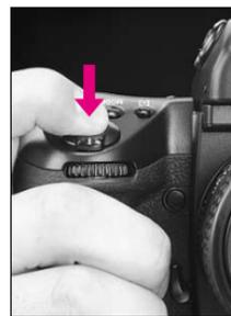
3 Compose picture, confirm focus and exposure, then fully depress shutter release button.
