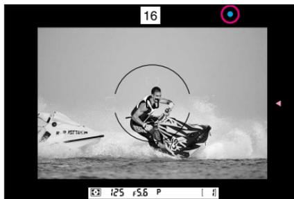
**With a moving subject:** Lightly press shutter release button to automatically activate Focus Tracking. Confirm ● appears in the viewfinder, then fully depress the shutter release button. (The shutter release button can in fact be depressed without confirming ● indication; as soon as the subject comes into focus, the shutter will be released.)
