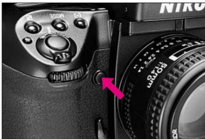
In Aperture-Priority Auto or Manual exposure mode, depress the depth-of-field preview button to stop the lens down to the aperture set with the Sub-Command Dial. In Programmed Auto or Shutter-Priority Auto exposure mode, the lens will be stopped down to the automatically set aperture. The viewed image becomes progressively darker as the aperture gets smaller. Those portions of the picture that appear in focus when the button is pressed are within the depth of field.
