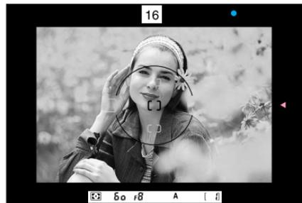
**3** Look inside viewfinder, compose and lightly press shutter release button. Confirm automatically set shutter speed.
