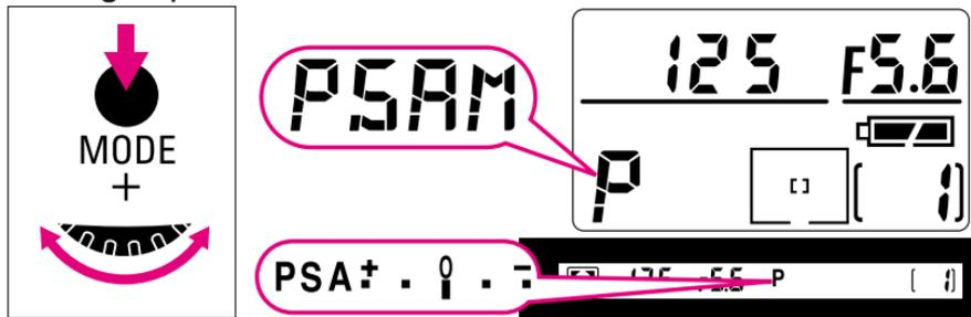
While pressing **MODE** button, rotate Main-Command Dial. The exposure mode changes as in the following sequence:
