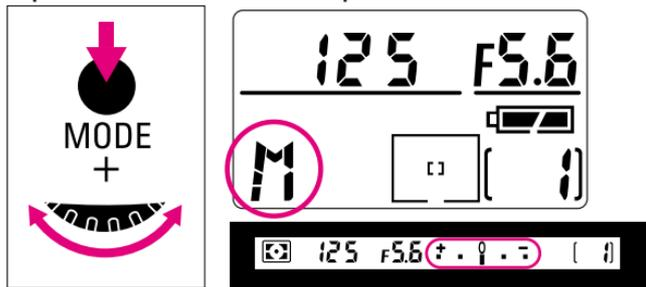
1 While pressing **MODE** button, rotate Main-Command Dial until **M** appears in the top LCD panel and electronic analog exposure display in the viewfinder.
