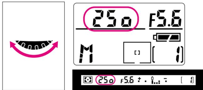
2 Remove finger from **MODE** button, set shutter speed by rotating the Main-Command Dial. Shutter speed can be set in 1/3 steps.
