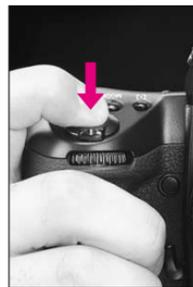
9 Confirm ● appears inside the viewfinder and fully depress the shutter release button to take the picture. The camera automatically advances the film by one frame, and LCD frame counter increases by one.
