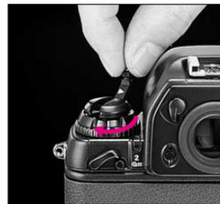
**1** To rewind film manually, press the film rewind button **1**
