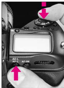
**2** Keeping shutter release button lightly pressed, confirm in-focus indicator ● appears in viewfinder. Then press and hold the AE-L/AF-L button to lock focus and exposure—and continue holding until step #3 is complete.
