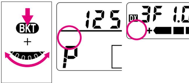
4 After the set number of shots has been taken, rotate the Main-Command Dial while pressing the **BKT** button so **BKT** disappears in the top and rear LCD panels to cancel Auto Exposure/Flash Exposure Bracketing. The number of shots and compensation value disappear when you remove your finger from the **BKT** button.
