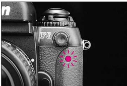
**3** Fully depress shutter release button. Self-timer LED starts blinking and shutter will be released after 10 sec. During the final two seconds, the LED lights up warning you to get ready for the shot.
