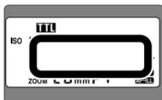
The flash shooting distance range disappears if the flash head is adjusted to other than the horizontal/front or down  $-7^\circ$  position.
