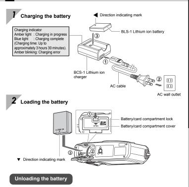
Turn off the camera before opening or closing the battery/card compartment cover.
