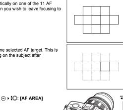
The camera focuses using one selected AF target. This is useful for accurately focusing on the subject after composing the shot.
