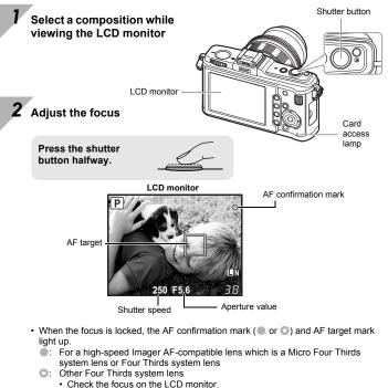
The shutter speed and aperture value that have been set automatically by the camera are displayed.
