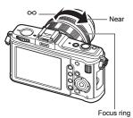
This function allows you to fine-adjust the focus manually by turning the focus ring after AF is performed in the S-AF mode.
