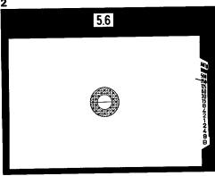
Exposure Compensation Warning. Whenever the automatic exposure is compensated by 1/4, 1/2, 2, or 4X, the aperture read-out changes from white to orange as a reminder, or warning (fig. 2).
