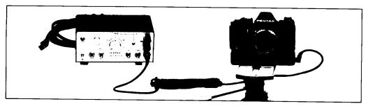
Off-Camera Remote Control: Shutter release for off-camera remote control with Power Pack M is controlled by the Power Pack shutter release button; the film advance mode is regulated by the Power Pack C/S switch.
