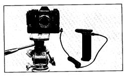
With Battery Grip M: When shooting with the camera mounted on a tripod or copy stand with battery grip M, the power source can only be used off-camera in conjunction with either the 3m (or 10m) Remote Control Cord.
