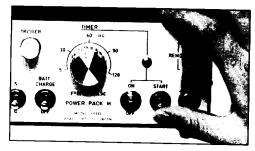
■ Set the timer start switch to START; the shutter will trip automatically after the predetermined interval elapses, the cycle repeating itself until the timer start switch is set to STOP, or to the end of the film.
