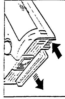
Insert the PC card into the PC Card Slot with the front surface of the card facing up. Push the PC card all the way into the slot until the edge of the card is flush with the PC card slot opening. If the PC card is properly inserted, [ EJECT ] appears on the LCD panel.
