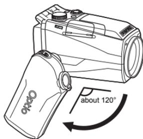
Rotate the grip to the desired position.
