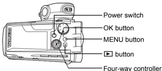
If the Initial Settings screen or Date Adjust screen appears when you turn the camera on, follow the procedure below to set the display language and/or current date and time.
