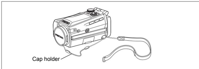
Attach the cap holder to the lens cap and thread the cord onto the camera strap. Remove the lens cap by pressing the tabs on either side of the cap.
