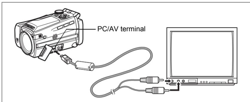
By using the AV cable, you can capture and play back images on a TV or other equipment with a video IN jack. Make sure that both the TV and the camera are turned off before connecting the cable.
