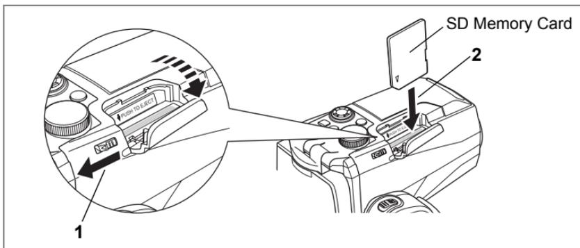
This camera uses an SD Memory Card to record captured images. Make sure that the camera is turned off before inserting or removing the SD Memory Card.
