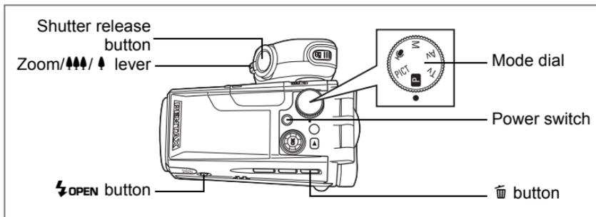
The standard procedure for taking still pictures is described below. If the flash has been opened, it will fire automatically depending on the light conditions.
