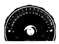
Select the shutter speed and f/stop combination desired from the top scales (11) and (12) on the calculator. Use this data to interpret the scene as described in the enclosed exposure system booklet.
