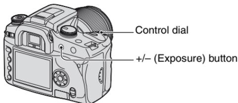
Press the +/- (Exposure) button and turn the control dial to adjust the exposure.
