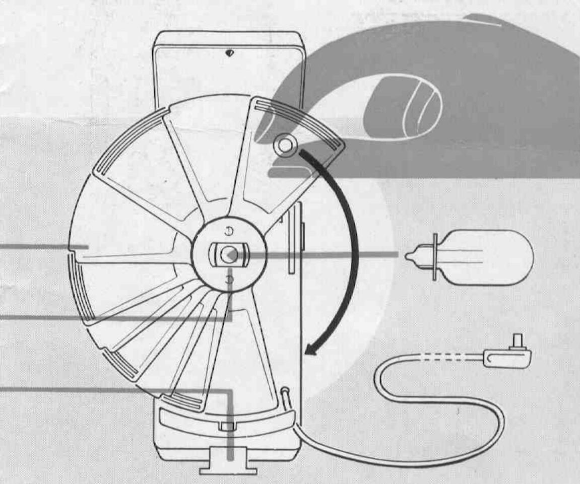
Inserting (and ejecting) the flash bulb: The flash gun is available in two models: for capless bulbs, and for bulbs with S.C.C. (BA 15s) or miniature pinless (American type M 2 and M 5) metal caps.
